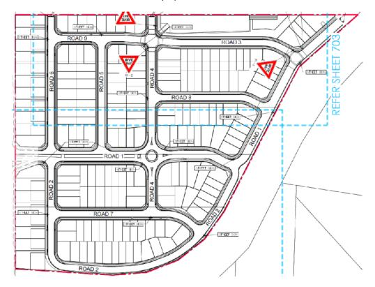
In addition to the roundabout, to reduce traffic speeds and conflict at the intersections of Roads 3/1 and 9/4, raised thresholds at the intersections with giveaway priority controls are proposed.
