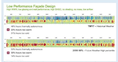
Figure 21: Modelled thermal autonomy for a minimally code-compliant apartment in Western Sydney, using both recent weather (TMY7 case) and predicted weather (2090 90% case) (Brannon 2018).
