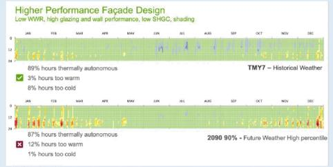
Figure 22: Modelled thermal autonomy for a high performance envelope apartment in western Sydney, using both recent weather (TMY7 case) and predicted weather (2090 90% case) (Brannon 2018).
