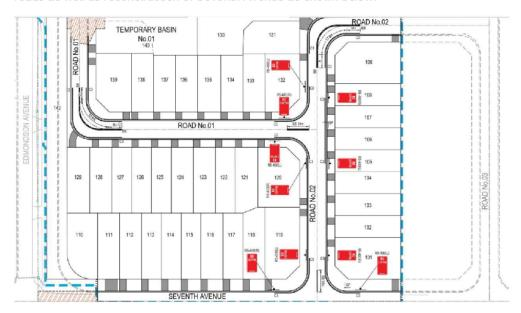
The road layout will result in two T-intersections and two 90-degree bends. The associated signs and linemarking scheme is as indicated above and is considered appropriate.
