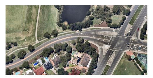
This section of Greenway Drive has a carriageway width of approximately 12m with a 2m raised concrete median island. The eastbound carriageway width is approximately 5m wide.
