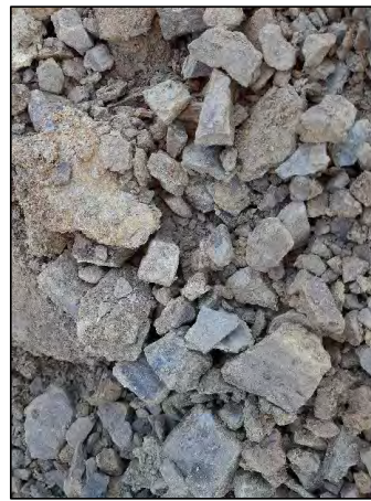
Photo Plate 13: Test pit TP5 – dark grey shale cobbles from 1.4 mBGL.
