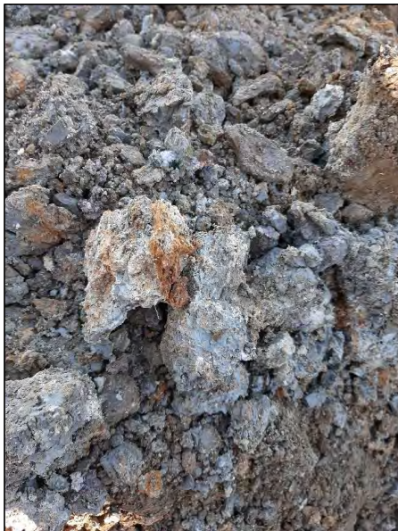
Photo Plate 9: Test pit TP3 – Orange and grey mottled clay from ~1.0 mBGL
