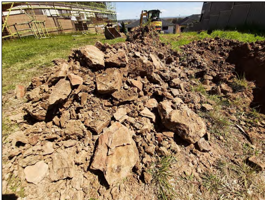
Photo Plate 18: Test pit TP10 – Excavated, large shale cobbles and boulders from 0.15 mBGL with quantity and size increasing with depth.
