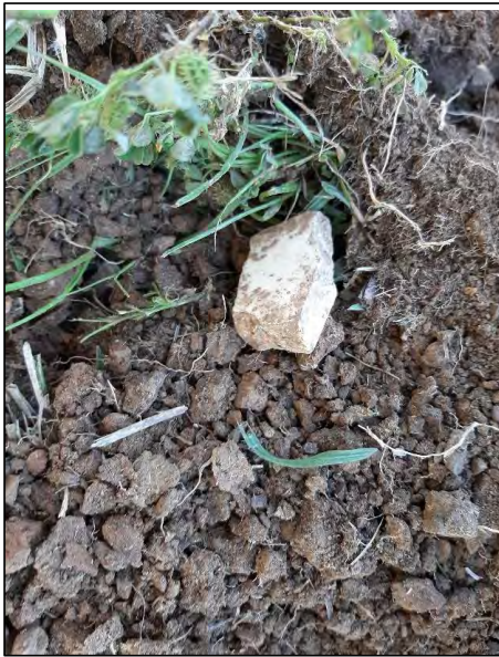
Photo Plate 15: Test pit TP7 – Trace inclusion of tile fragment within shallow fill.
