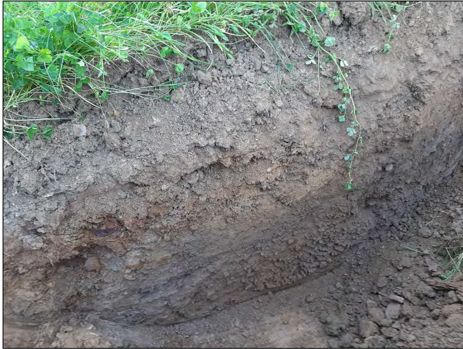
Photo Plate 11: Test pit TP5 – Shallow fill overlaying orange and grey mottled clay with shale cobbles at depth
