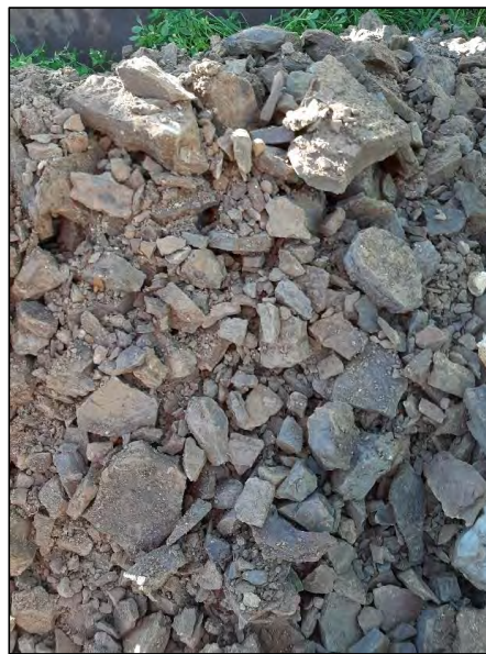
Photo Plate 10: Test pit TP3 – Brown and dark grey shale cobbles from ~1.4 mBGL.
