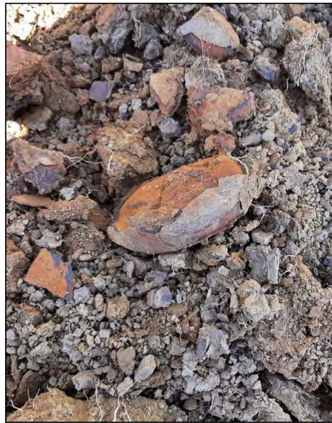
Photo Plate 16: Test pit TP7 – Large, brown and dark grey shale cobbles from ~1.4 mBGL.
