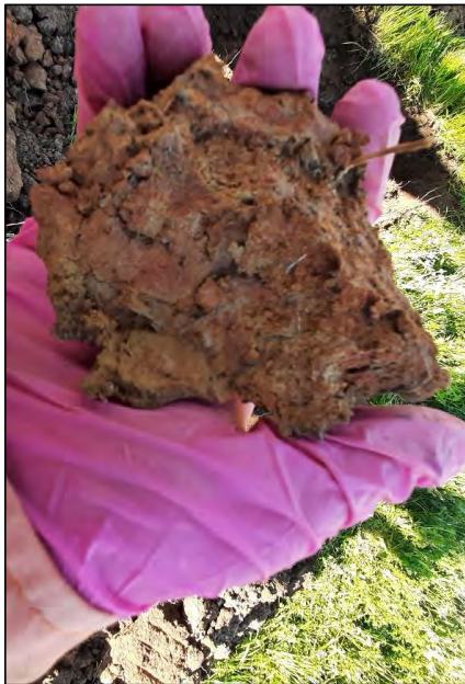
Photo Plate 4: Test pit TP1 – Natural mottled red and beige clay from ~0.5 mBGL.
