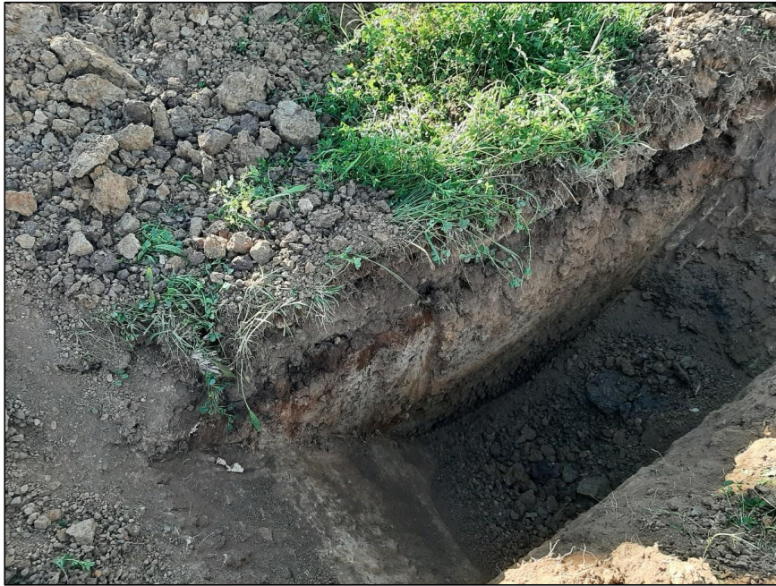
Photo Plate 6: Test pit TP2 – Shallow fill overlaying natural mottle orange and grey clay with shale cobbles from ~1.0 mBGL.
