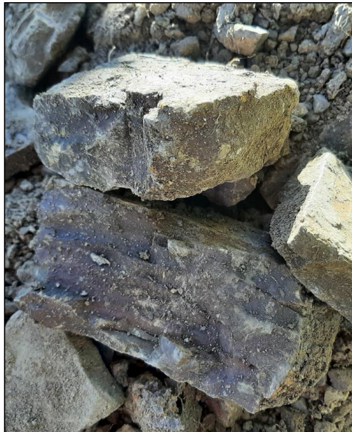
Photo Plate 5: Test pit TP1 – Natural dark brown/ grey shale cobbles from 0.9 mBGL.
