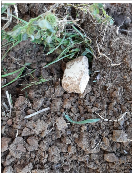
Photo Plate 15: Test pit TP7 – Trace inclusion of tile fragment within shallow fill.
