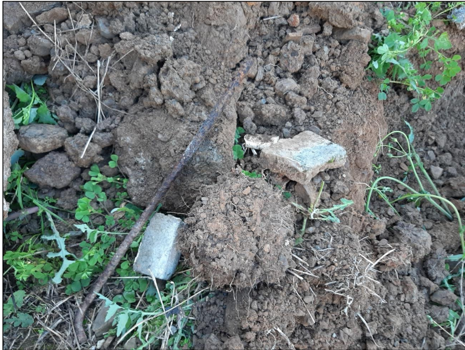
Photo Plate 8: Test pit TP3 – Brown clay from 0 – 0.5 mBGL with inclusions of trace brick and tile fragments and metal rod.
