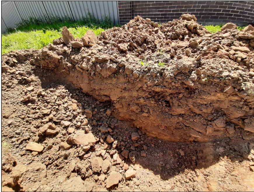
Photo Plate 17: Test pit TP10 – Shale cobbles and boulders from 0.15 mBGL.
