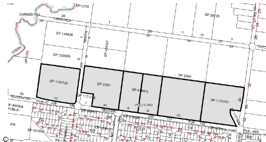
Figure 7: Speed humps are to be provided within the service road to be located on the highlighted lots at 100m intervals.
