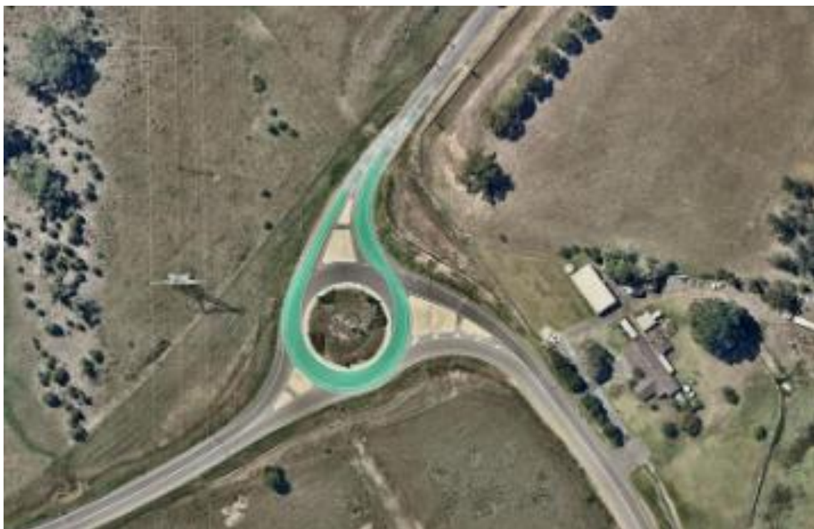
Figure 2: Swept path analysis for A-Double Truck movement
